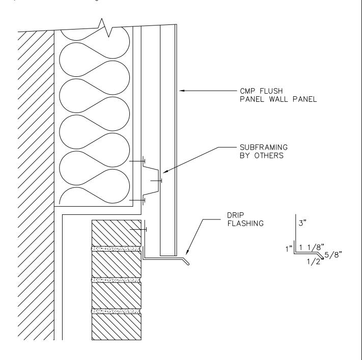
DETAIL: Drip Edge @ Wall SYSTEM: CMP Flush Panel
